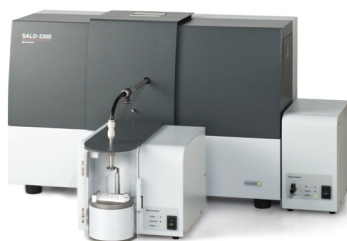
Dry Measurement System (SALD-2300 and SALD-DS55)
